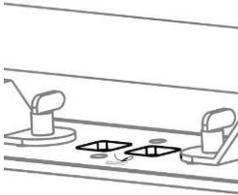
Fasten a safety cable (not shown) between the support structure and the attachment point on the fixture. The safety cable must be able to bear at least 10 times the weight of the fixture.
