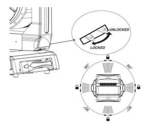
The X-axis rapid lock forward is LOCKED, and backward (UNLOCKED) to open.
