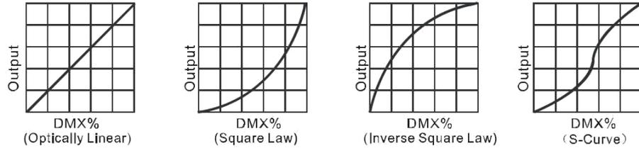
**Linear:** The increase in light intensity appears to be linear as DMX value is increased.
